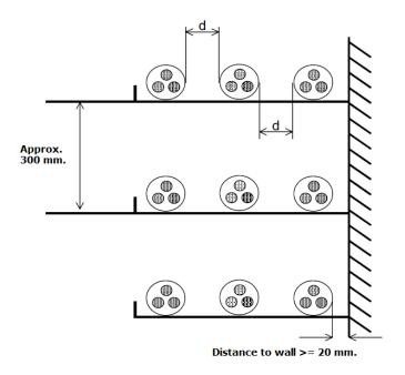
b) Three-pole cables or triplets of single-pole cables lying on perforated cable trays, separated each other a distance of one diameter (d), as per IEC 60287:
