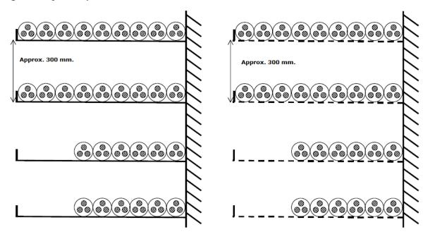
e) Three-pole cables or triplets of single-pole cables in contact between them, lying on a structure or wall, as per IEC 60287:
