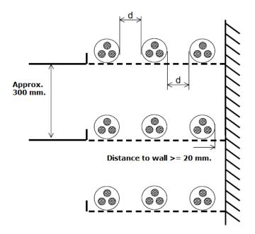
c) Three-pole cables or triplets of single-pole cables lying on structures or walls, separated each other a distance of one diameter (d), as per IEC 60287:
