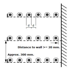
i) Single-pole cables lying on a structure or wall at a distance (D) of at least 20 mm., one over the other, with separation between them equal to a diameter (d), as per IEC 60287:
