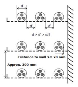
g) Single-pole cables lying on continuous trays (restricted airflow) with separation between them equal to a diameter (d), as per IEC 60287:
