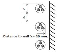
d) Three-pole cables or triplets of single-pole cables in contact between them and with the wall, lying on trays (where the airflow is restricted), as per IEC 60287:
