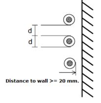
j) Single-pole cables lying on a structure or wall at a distance smaller than 20 mm., one over the other, with separation between them equal to a diameter (d), as per IEC 60287:
