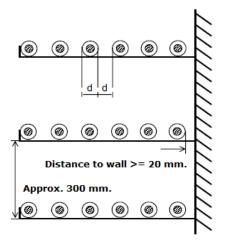
h) Single-pole cables lying on perforated trays with separation between them equal to a diameter (d), as per IEC 60287:
